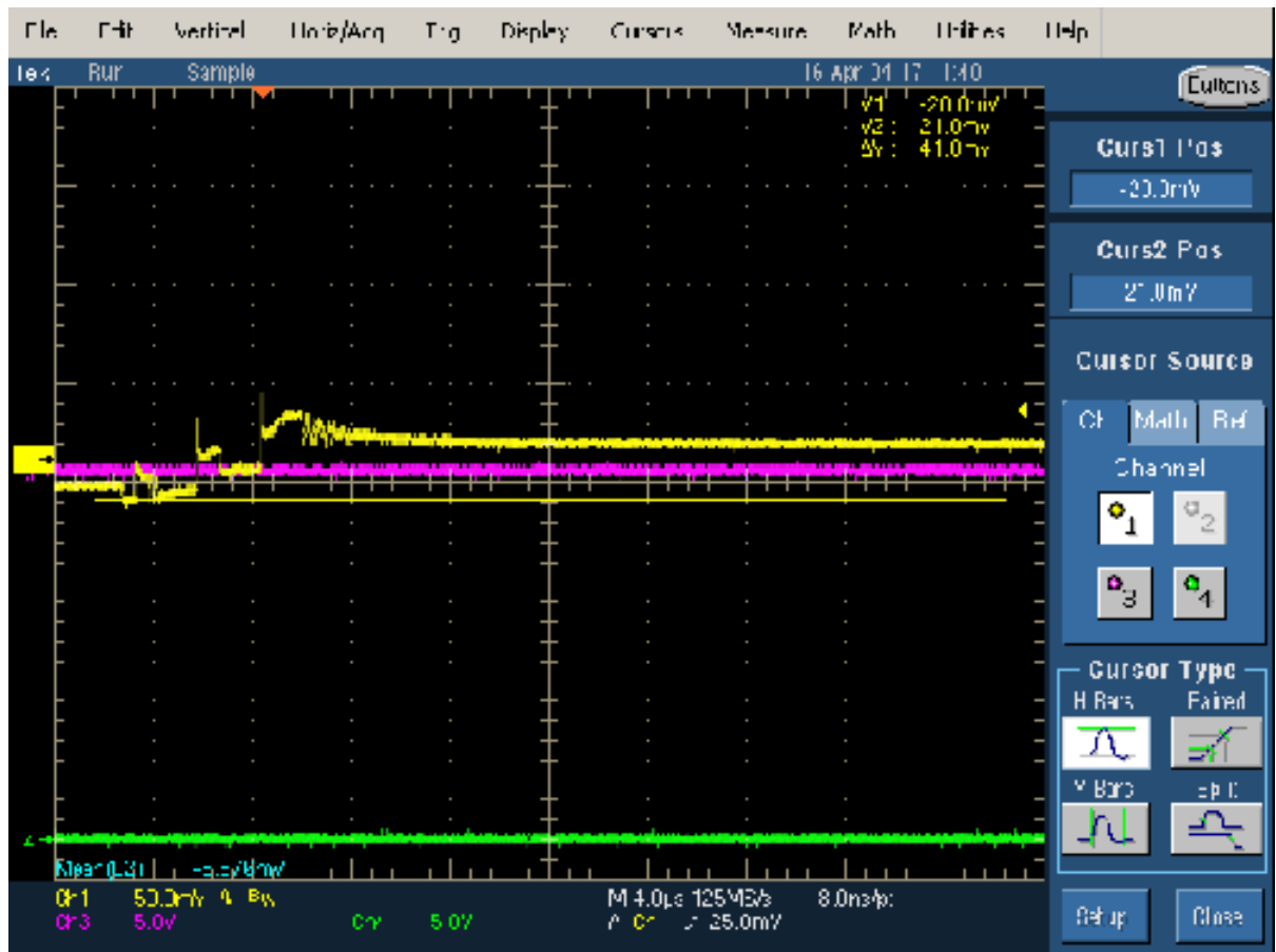
FIGURE 9. Feedback pin for V_{in}=2.7V and I_{out}=0A
